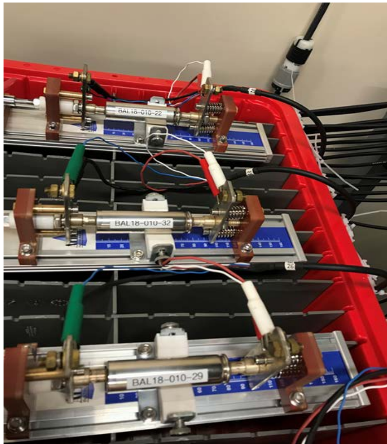
Figure 4 : Several 2170 cells undergoing performance and supply chain qualification process.
