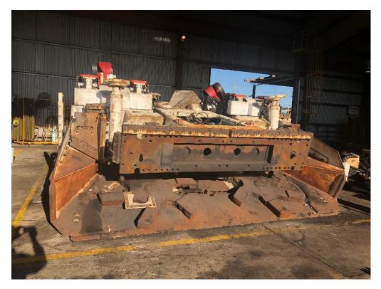
Fourth continuous miner to go underground at end of July, awaiting final fitting of the cutter head.
