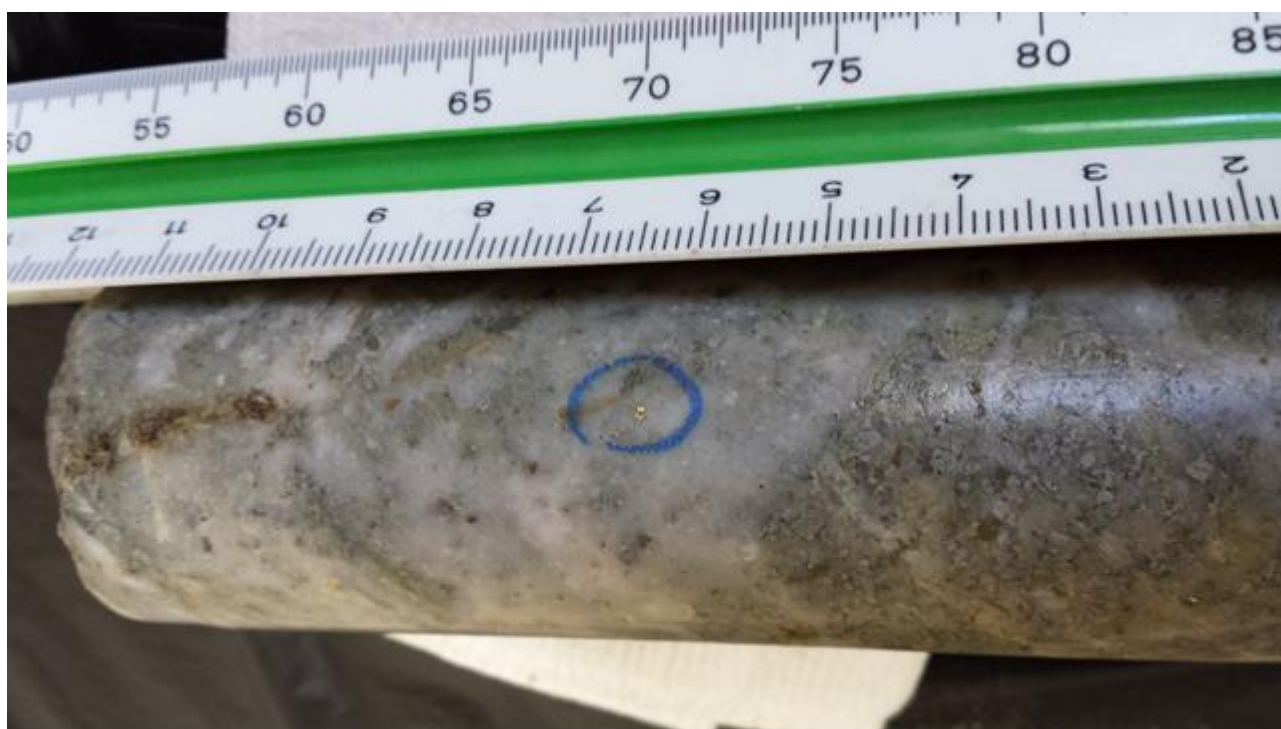
Photo 2. Visible gold in altered dyke in drillhole L7016, at 44.15 m down hole.
