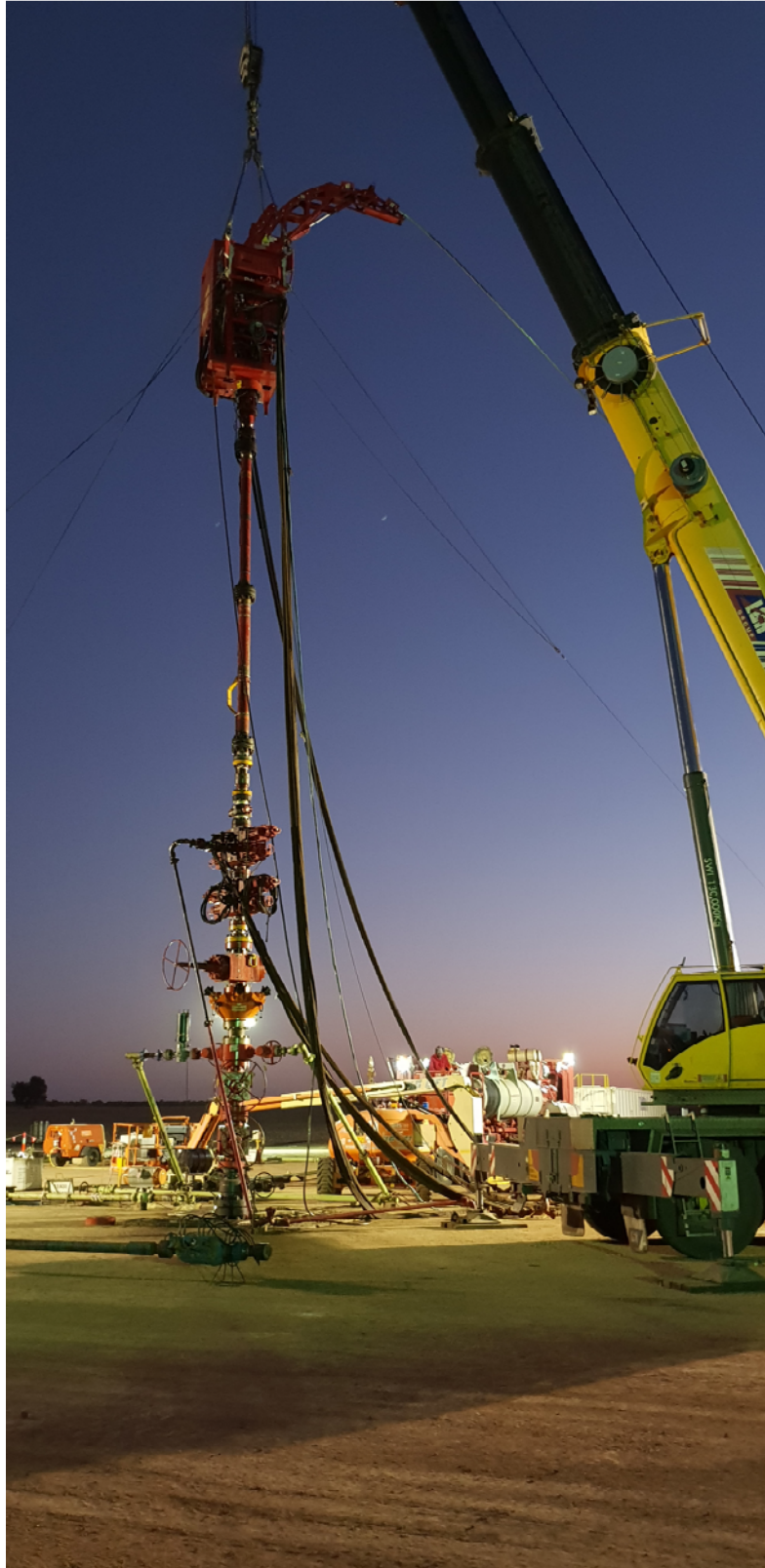
Coil unit set up while milling out plugs after hydraulic stimulation
