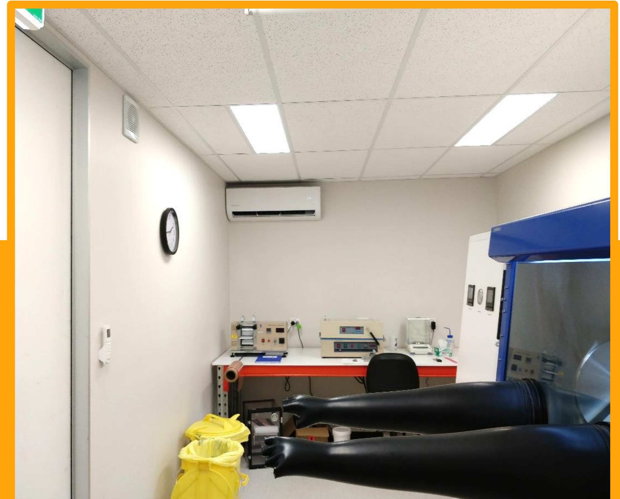
Internal battery lab capable of: slurry mixing, electrode coating, cell assembly and testing
