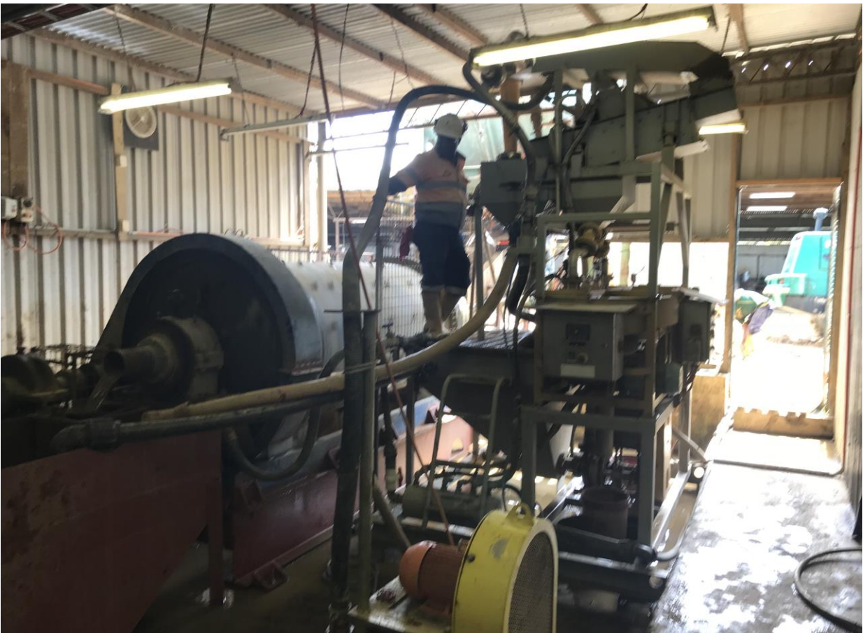
Eddie Creek Processing Manager and Metallurgist, Joma Mering, overseeing the milling and ISP concentrator operations
