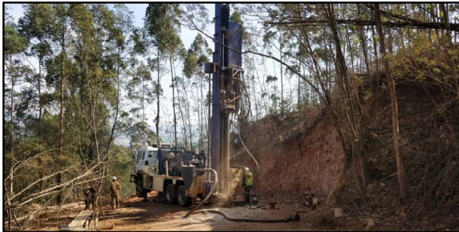
Figure 5: RC-rig No.2 infill drilling at Theta Hill (DG4 area)
