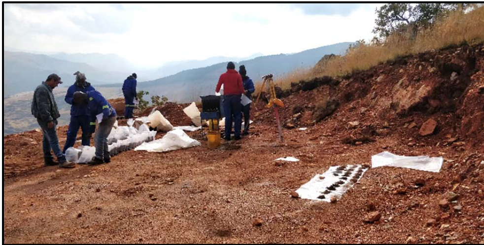
Figure 6: Sampling underway of RC chips at Theta Hill RC Rig No.1 (August, 2018)
