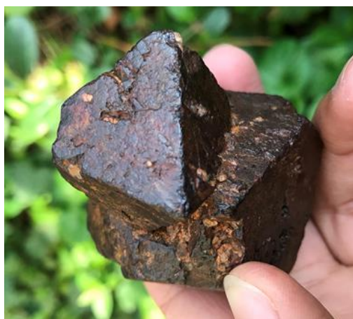
Picture 1a – Hematite (iron oxide) pseudomorph after pyrite collected from Sidewinder Prospect (indicative hand-held XRF values of 0.26% copper and 0.33% cobalt).
