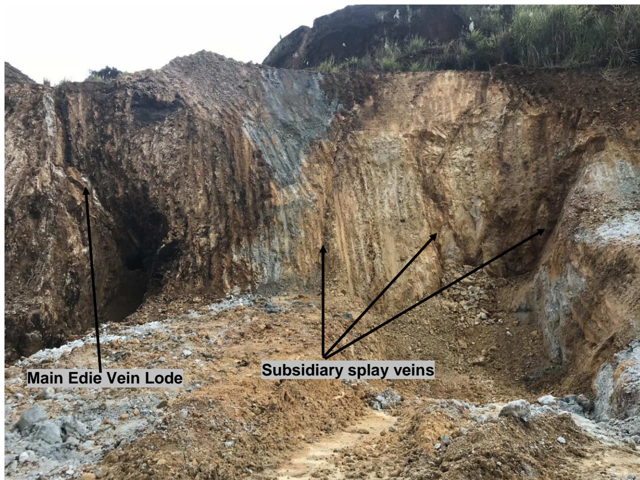
Figure 9: The current top bench showing the main Edie Lode (dark on left) and splay veins (right)
