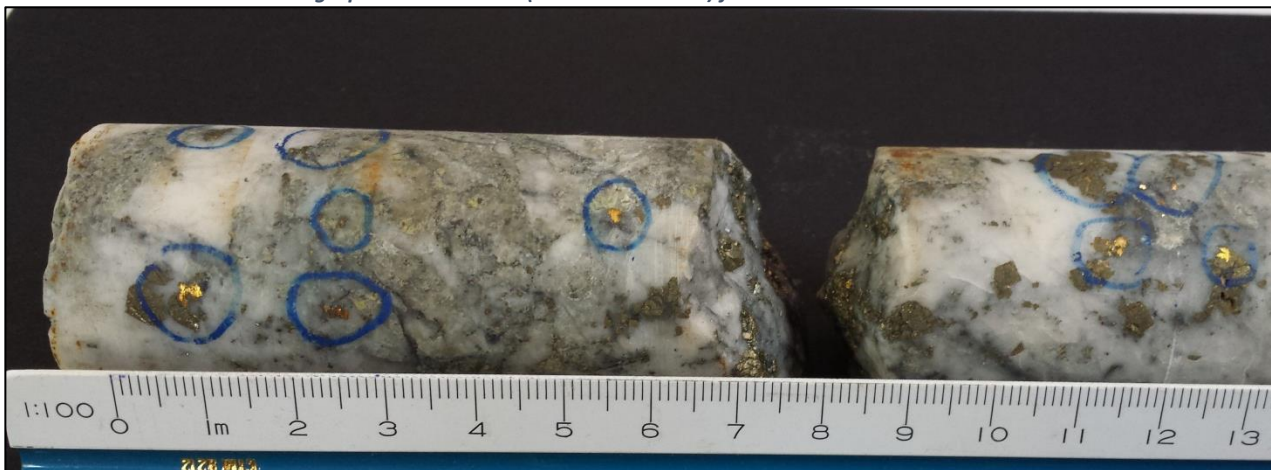
Photograph 1: Visible Gold (inside blue circles) from 42.70m. Drill hole L7029.
