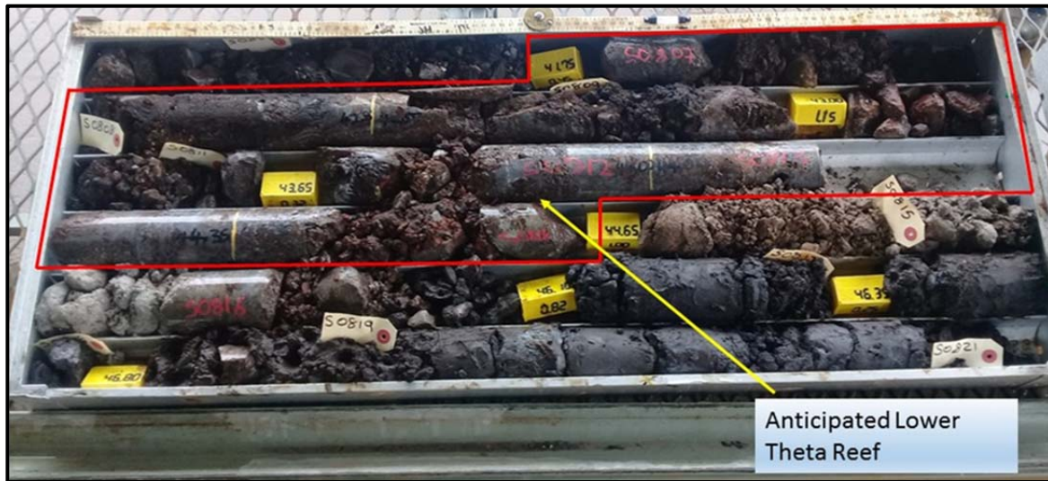
Figure 2) Example of weathered drillcore
