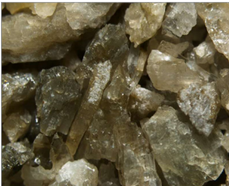
Test work Comp P100 5.6mm +0.5mm DMS100 SG 2.9 Overflow P100 3.35mm +0.5mm DMS100 SG 2.9 Underflow
