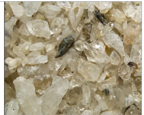
Test work Comp P100 5.6mm +0.5mm DMS100 SG 2.9 Overflow P100 3.35mm +0.5mm DMS100 SG 2.7 Overflow
