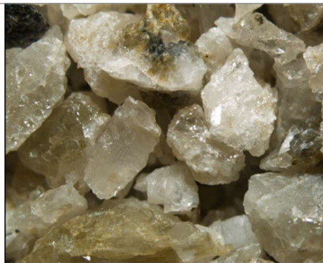
Test work Comp P100 5.6mm +0.5mm DMS100 SG 2.9 Overflow P100 3.35mm +0.5mm DMS100 SG 2.9 Overflow
