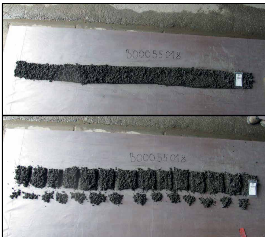
Photo 8-4: Example of Sample Splitting by the Wet Japanese Slab Cake Homogenization Method
