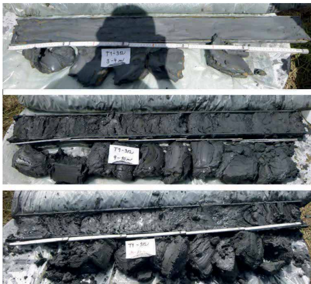
Photo 8-2: Core Photos from Drill Hole T1-312, from Depths 3-4 m, 9-10 m and 23-25 m
