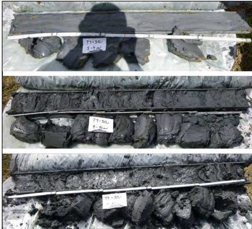
Photo 1-1: Core Photos from Drill Hole T1-312, from Depths 3-4 m, 9-10 m and 23-25 m
