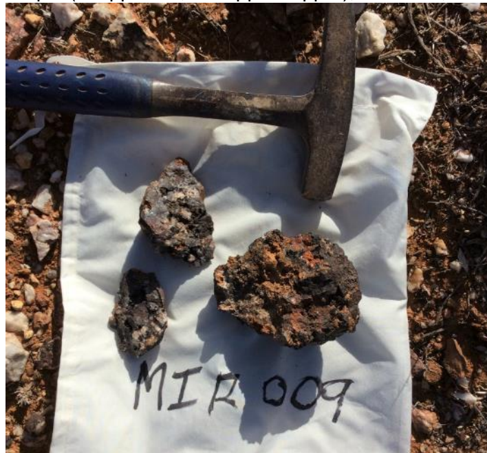
Plate 3: Benco gossan sample (188ppm Co, 3040ppm copper), 578863E, 6484446N
