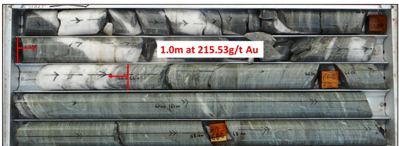
Figure 4: NADD004- Silicification and quartz veining in extreme high-grade diamond drill core
