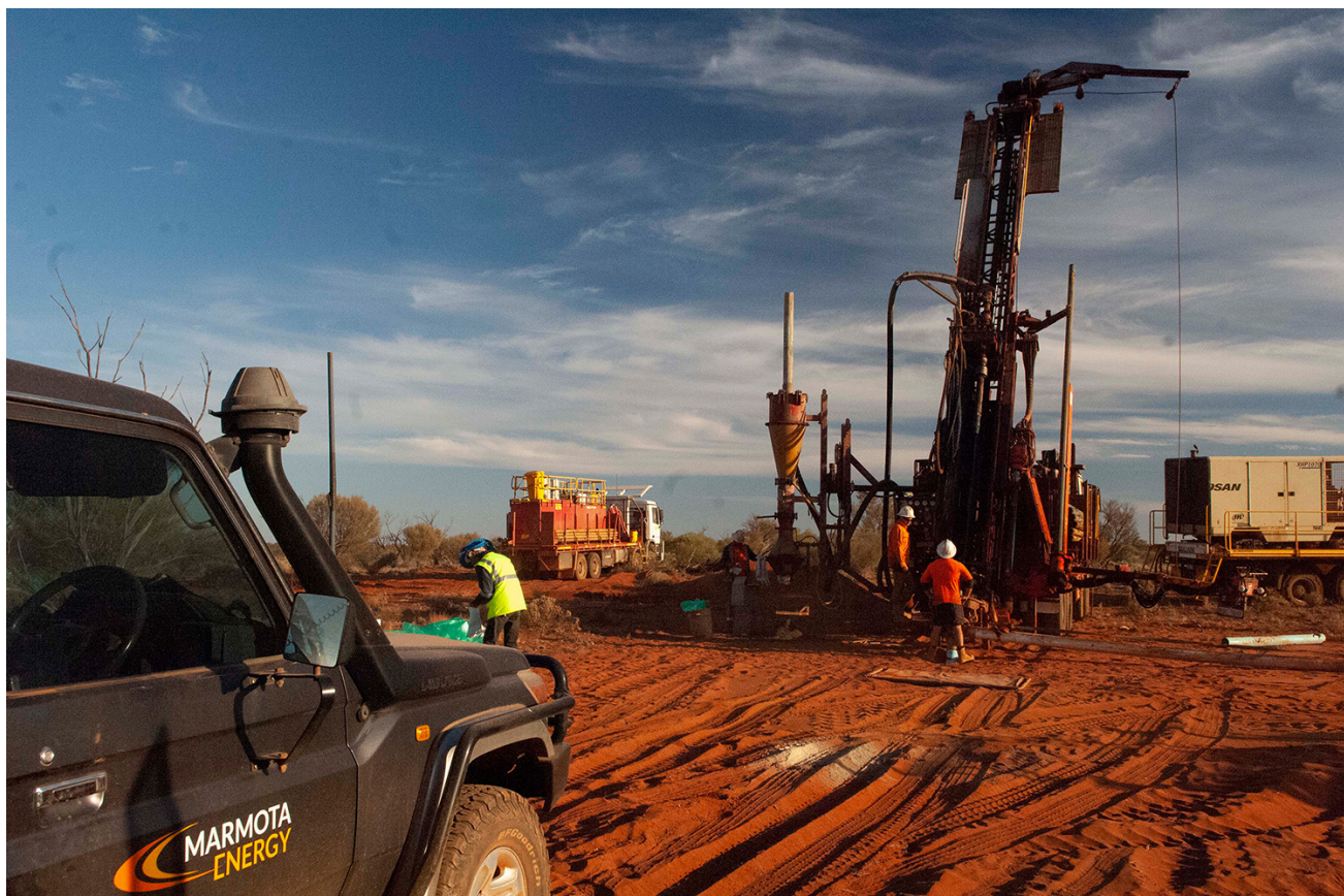
Figure 7: Aurora Tank during May 2018 drilling program with Bullion Drilling Co RC rig
