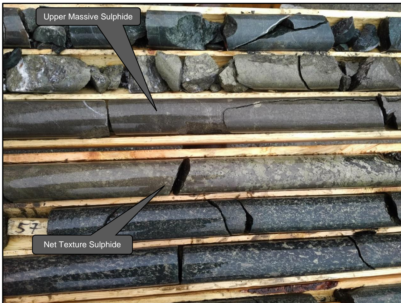
Figure 6: ZA-18-04 – upper massive sulphide and 20-30% net textured sulphides at 57m
