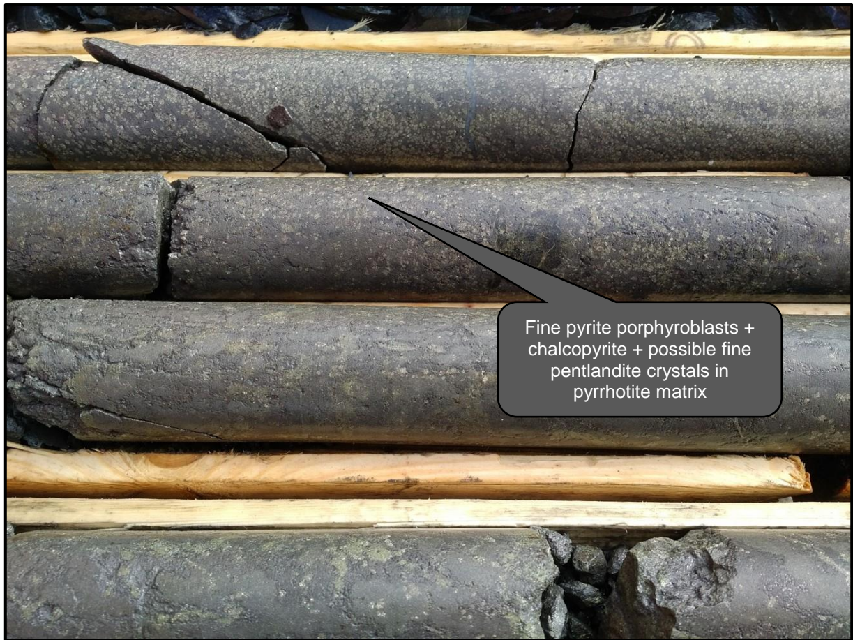
Figure 12: ZA-18-08 - massive pyrrhotite-pyrite zone from 86m
