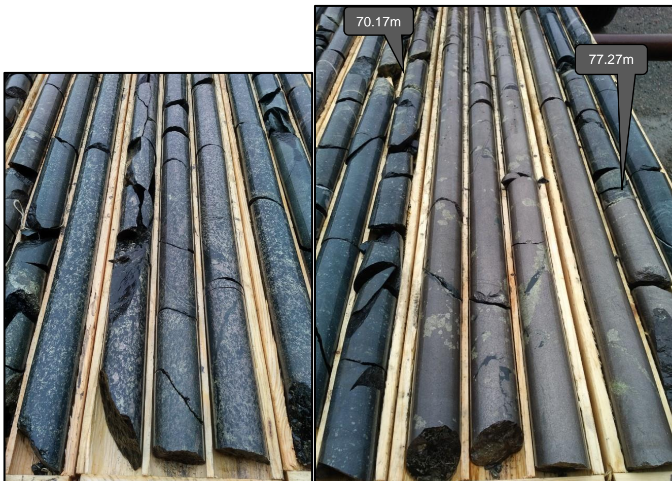
Figure 8: ZA-18-04 with 20-30% net texture sulphides ~60m (left) and the lower massive sulphide from 70.17m
