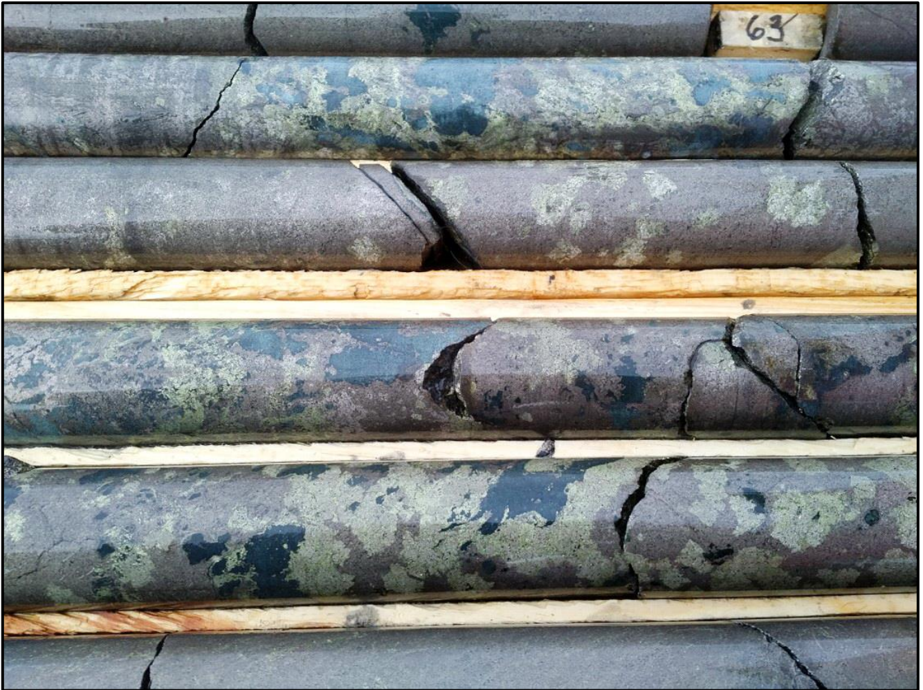
Figure 10: Hole ZA-18-05 – massive sulphide from 63m, remobilised/brecciated pyrrhotite-pyrite - chalcopyrite with chlorite inclusions (dark green)
