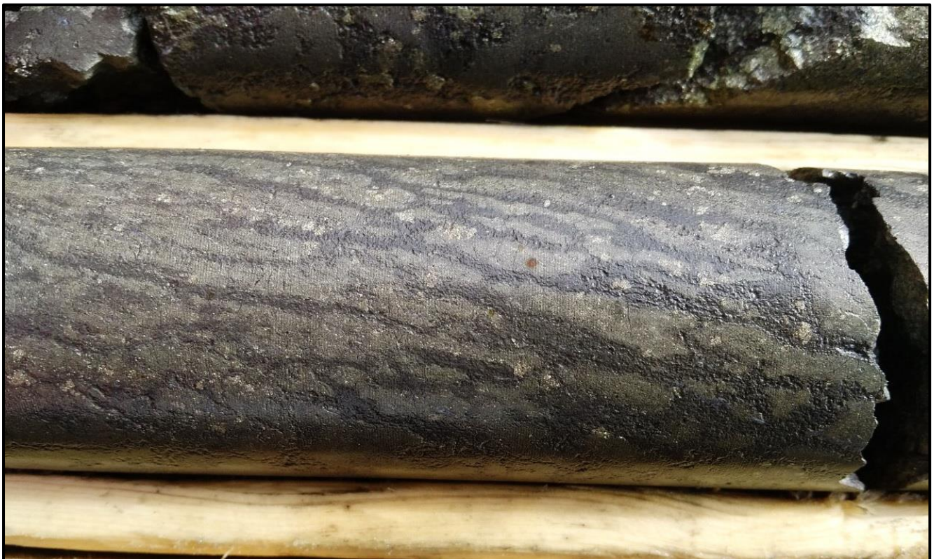
Figure 13: ZA-18-08 – laminated pyrrhotite-pyrite zone at 92.8m
