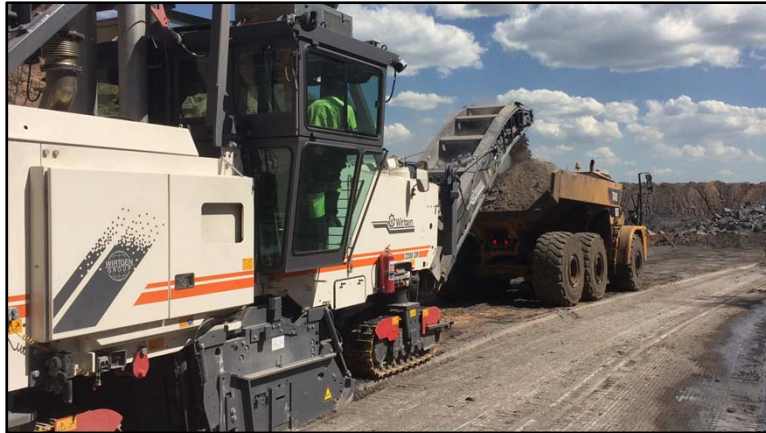
Example of Surface Miners which can be applied to open cut mining.
