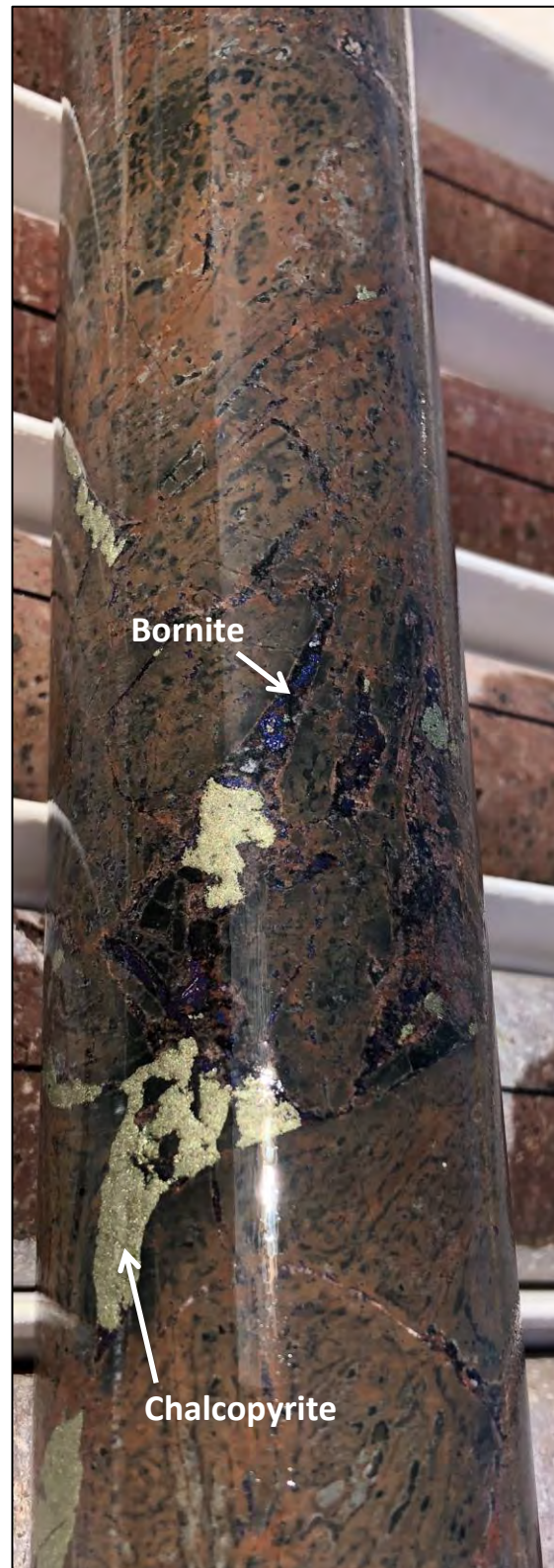
[Figure 2] Punt Hill: DD18PTH001 core photograph showing strong retrograde K-feldspar-chlorite alteration and replacement of prograde garnet skarn with associated chalcopyrite-bornite stockwork from 833-834 metres.
