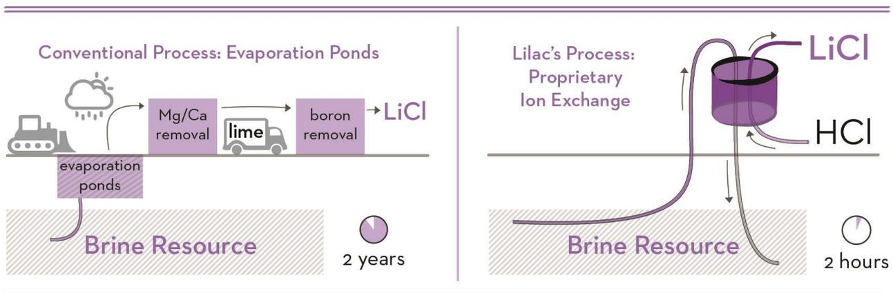
**Figure 1. Conventional Process for lithium extraction of brines from evaporation ponds (left) versus Lilac’s innovative Ion Exchange method (right), which promises high recoveries in a few hours versus 9-24 months using evaporation to concentrate the lithium. Lilac’s method allows for the re-injection of brines to the aquifer from where it is sourced without significantly adjusting the water quality.**
