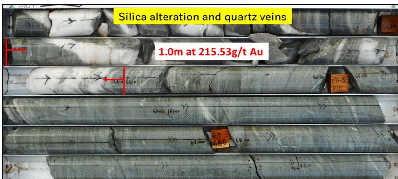
Figure 5: NADD004- Silicification and quartz veining in extreme high-grade diamond drill core
