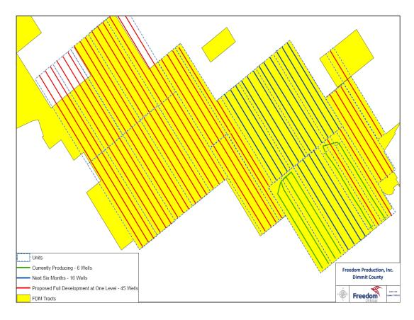
The attached development map shows the area of our field development for the next year or more. The six locations marked in green are our currently producing wells. The 16 locations in blue are the firm locations we are drilling now and will continue to drill over the six months of our current drilling rig contract which ends in February 2019.
