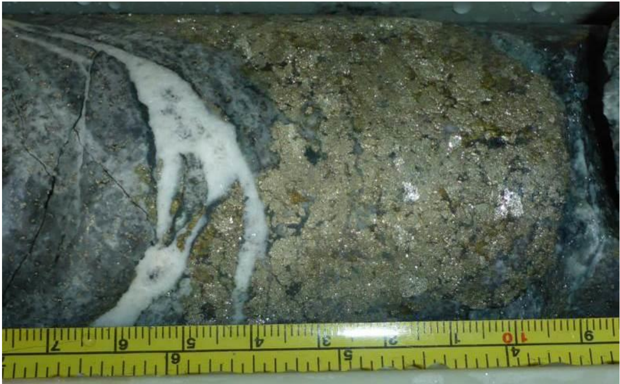
Figure 8. MCD001 - 273.7 metres downhole. Quartz -pyrite-chalcopyrite vein in altered diorite
