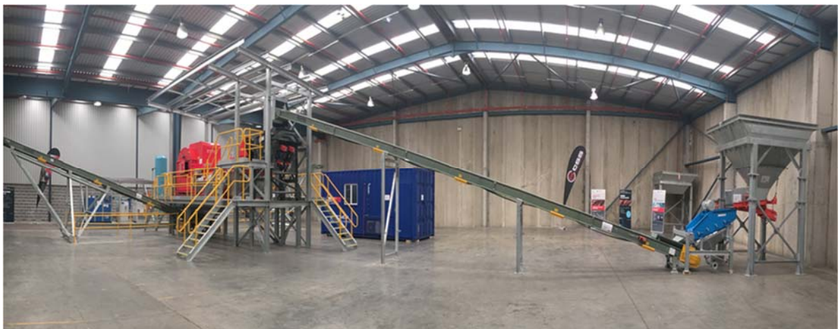
Figure 2: TOMRA 1200 XRT Ore Sorter and ancillary equipment
