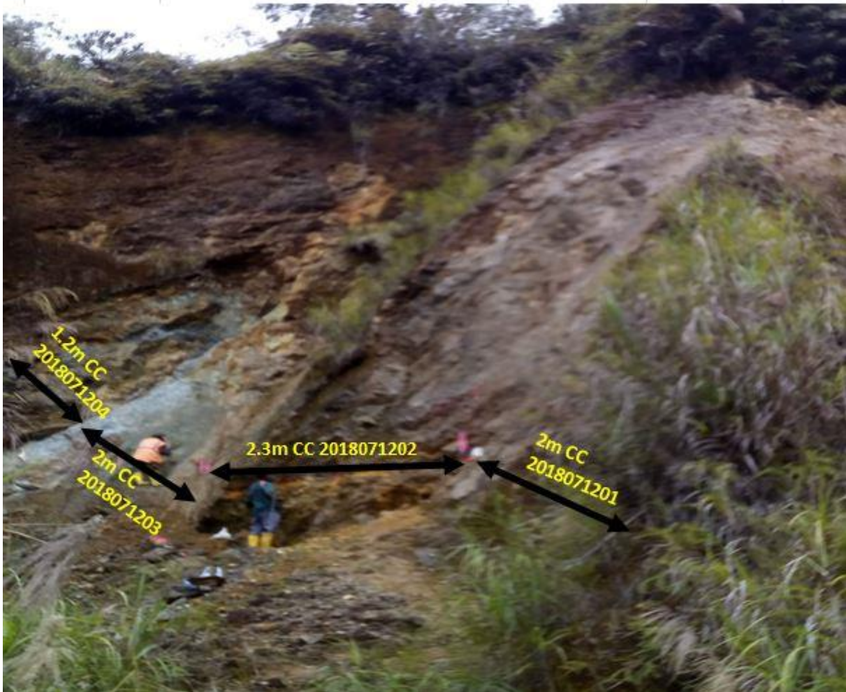
Figure 3: Karuka South outcrop showing continuous channel sample lines. Left hand samples 1 and 2 are vein outcrop and 3 and 4 are puggy alteration channel samples.
