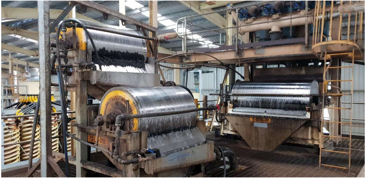
Photo 4. LIMS removing the titano-magnetite
