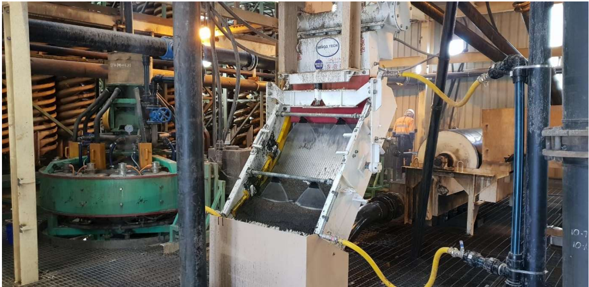
Photo 3. New sieve bend in action
