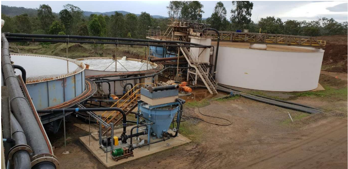
Photo 5. Thickeners removing the slimes
