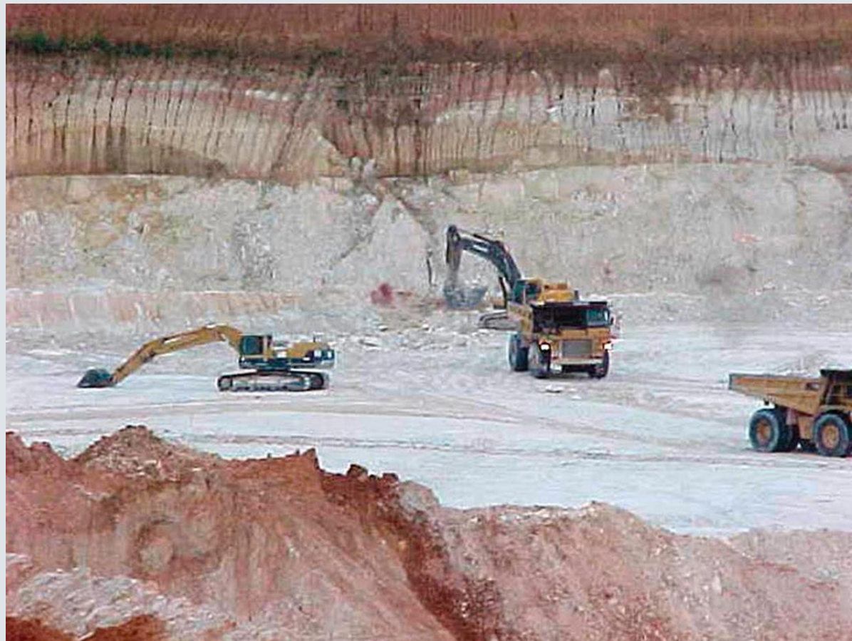
Typical Dry Mining Kaolin Operation
