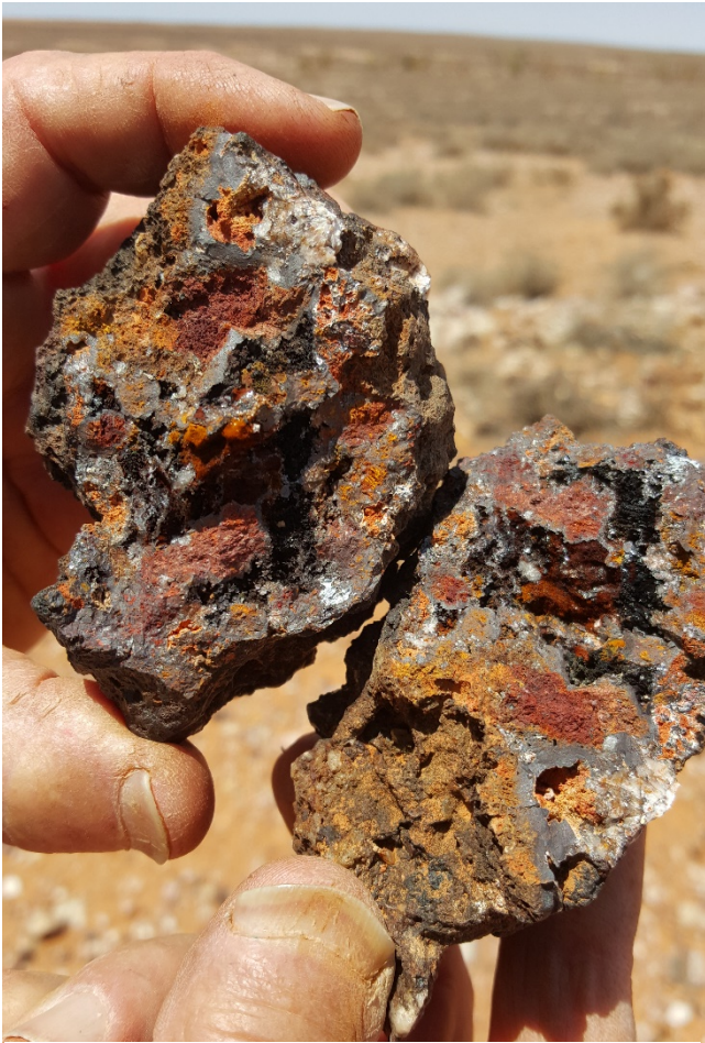
Plate 1: Benco prospect gossanous quartz iron oxide vein sample (578863E, 6484446N)
