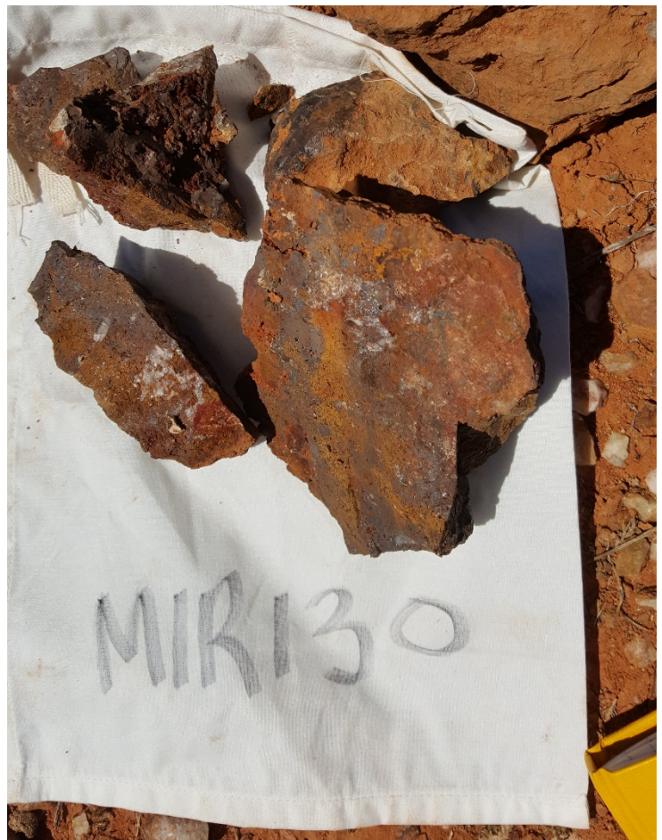
Plate 2: MIR130 Quartz iron oxide vein (3520ppm Cu and 0.3g/t Au) (578096E, 6483908N)
