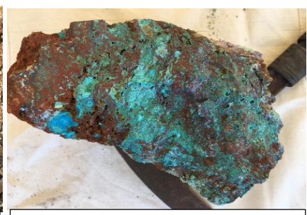
Photo 3. Outcrop adjacent black shale adjoining Black Shale unit, 2 km south of LD18RC006. 33.40 g/t Au, 32.70% Cu, 1,610 ppm Co. (Refer ASX Release 6 th December)
