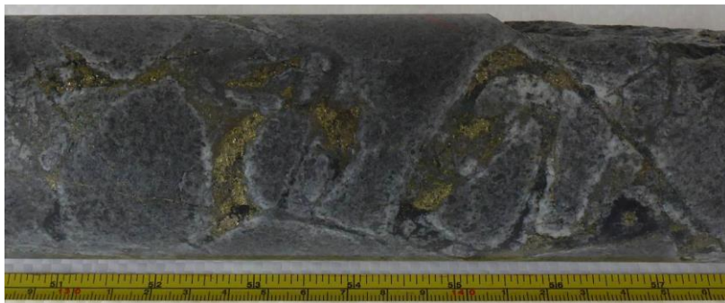
MCD002, 189.80-189.98m: Brecciated tonalite with chalcopyrite, pyrite, magnetite (black) and quartz cement (HQ Core 63mm diameter; scale: inches and centimetres)
