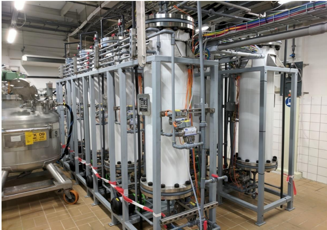
Chromatographic Separation Unit installed at BPF
