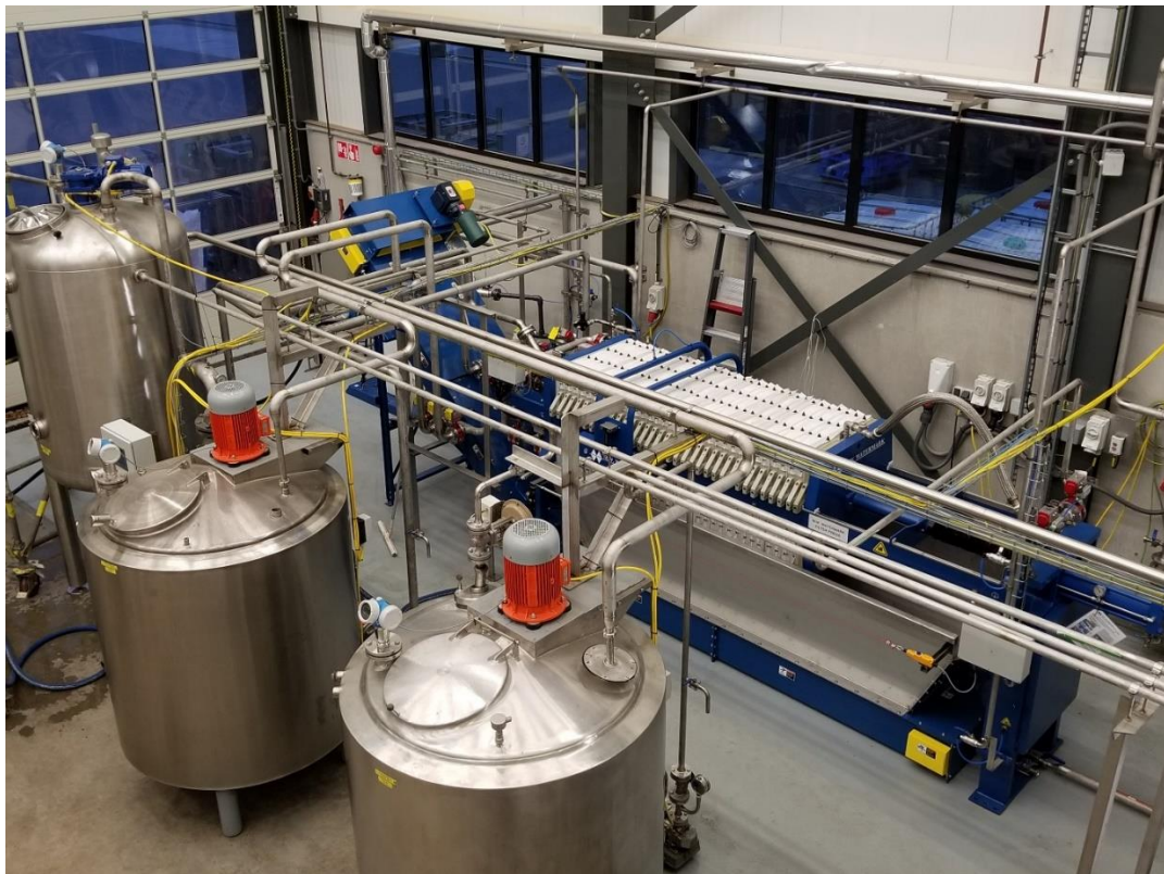
Automated Membrane Press Filtration Unit installed at BPF
