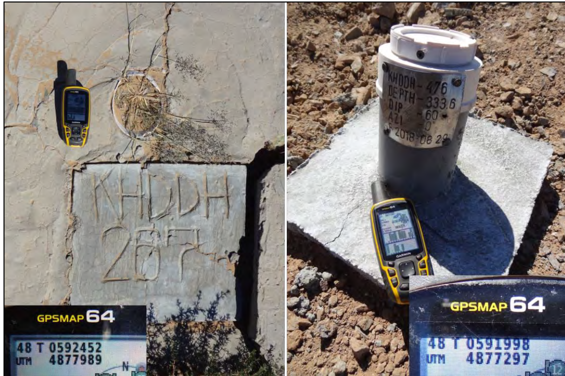
Figure 38: GPS confirmation of additional drillhole collars by CSA Global
