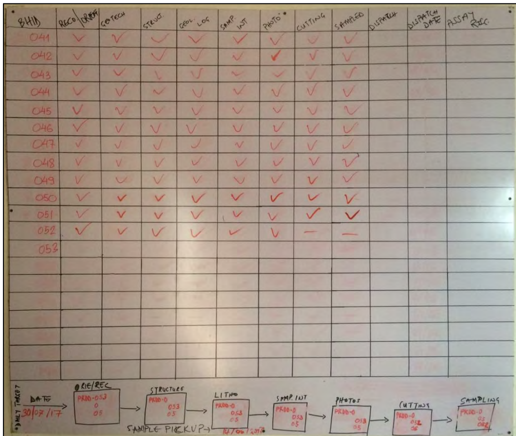
Figure 40: Whiteboard tracking of steps in core handling process
