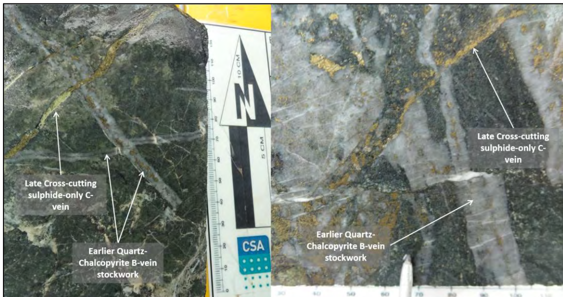
Figure 20: Late sulphide-only C-veins overprinting earlier quartz-sulphide B-veins
