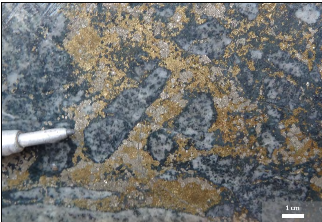
Figure 22: Pyrite-chalcopyrite cemented hydrothermal breccia
