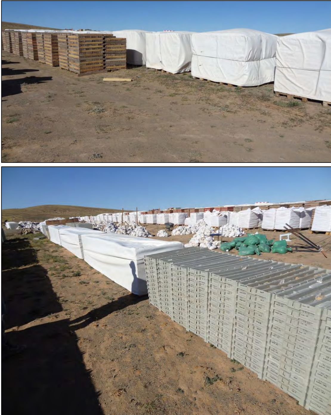
Figure 35: Drill core storage farm where most drill core stacks are protected by purpose-made covers
