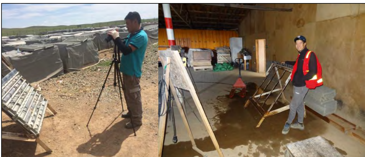
Figure 42: Core photography setup: Pre-2018 natural light photography (left) current controlled lighting indoor photography frame (right)
