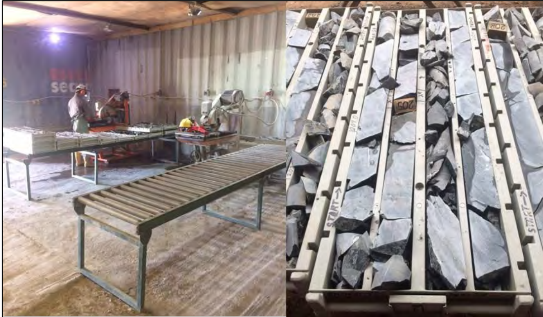
Figure 43: Core cutting area (left) and cut core ready for sampling (right)
