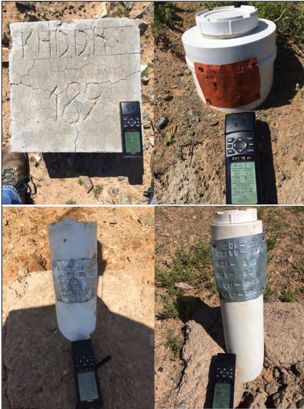
Figure 37: GPS confirmation of drillhole collar positions validated by Mining Associates (MK1715 2018)
