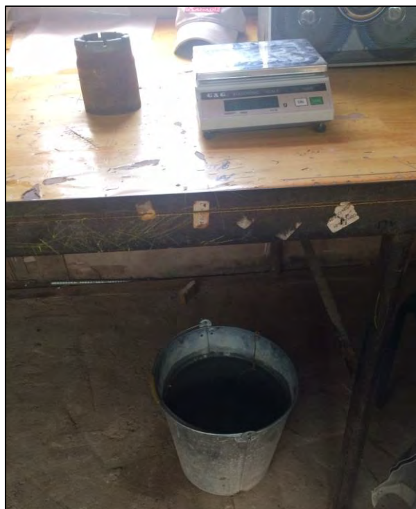
Figure 45: Apparatus for specific gravity measurements
