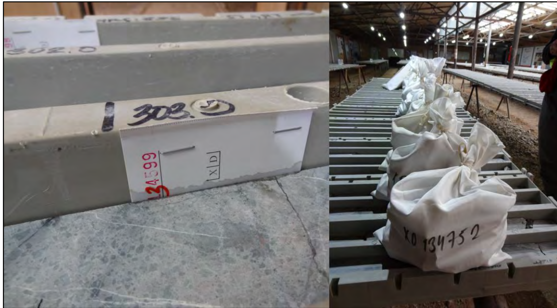
Figure 44: Drill core sampling; sample tags stapled into core trays (left), sample bagging and numbering (right)
