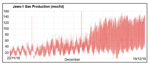
Strike continues to manage the reservoir drawdown carefully to ensure the maximum volume of coal remains in communication with the well and enters the desorption window. Water production remains stable which indicates that continued fluid recovery will yield material gas production growth. Pump speed has been kept flat throughout this period with bottom hole pressures only reducing a few PSI per day.
