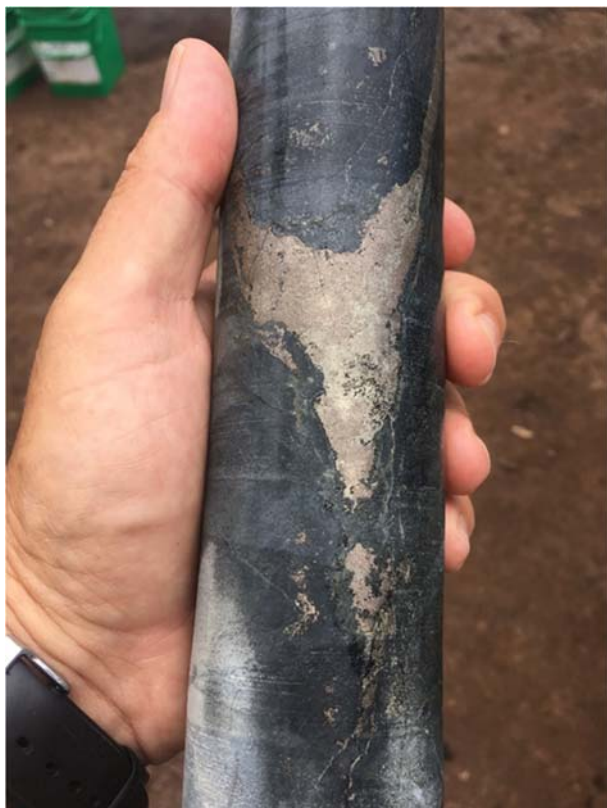
Figure 2 – Sulphides observed in Pembroke core (PEM029, depth 388m)
