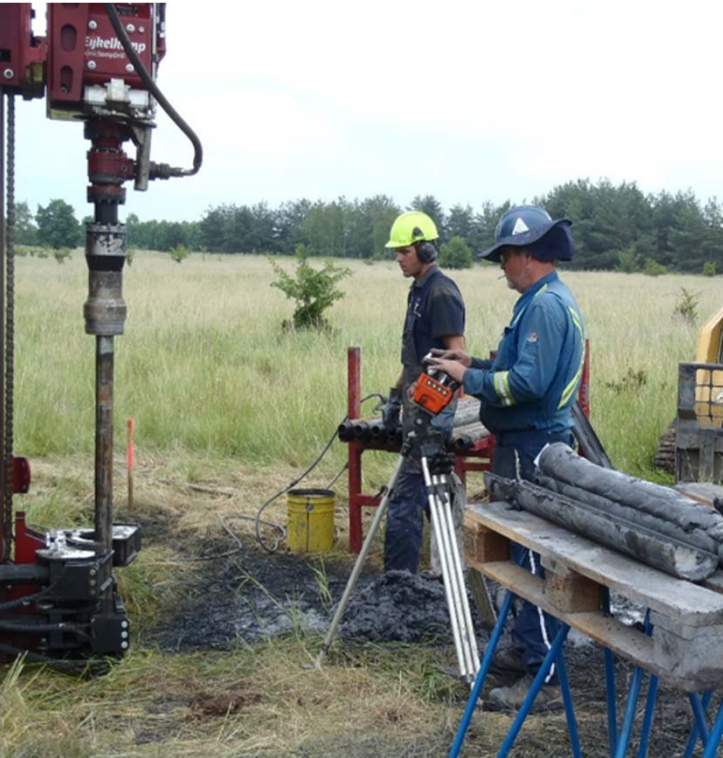
↑ Sonic drill – modern, effective sampling tool
