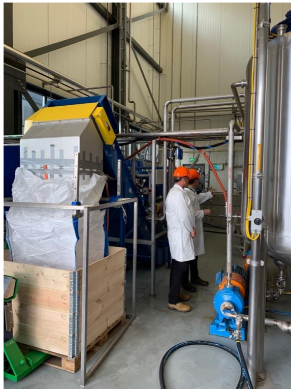
Solids separation with the plate and frame filter unit and associated operations integrated at BPF.
