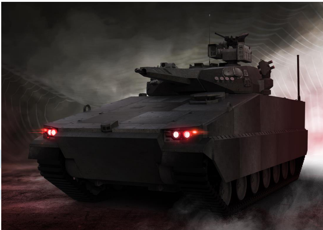
The Hanwha “Redback” infantry fighting vehicle featuring the EOS T-2000 turret and R-400S remote weapon station mounted above the turret
