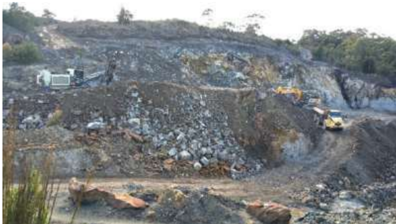
Figure 1 – Mining activities at the Granville East Mine (showing cut-back progressing on eastern wall)
