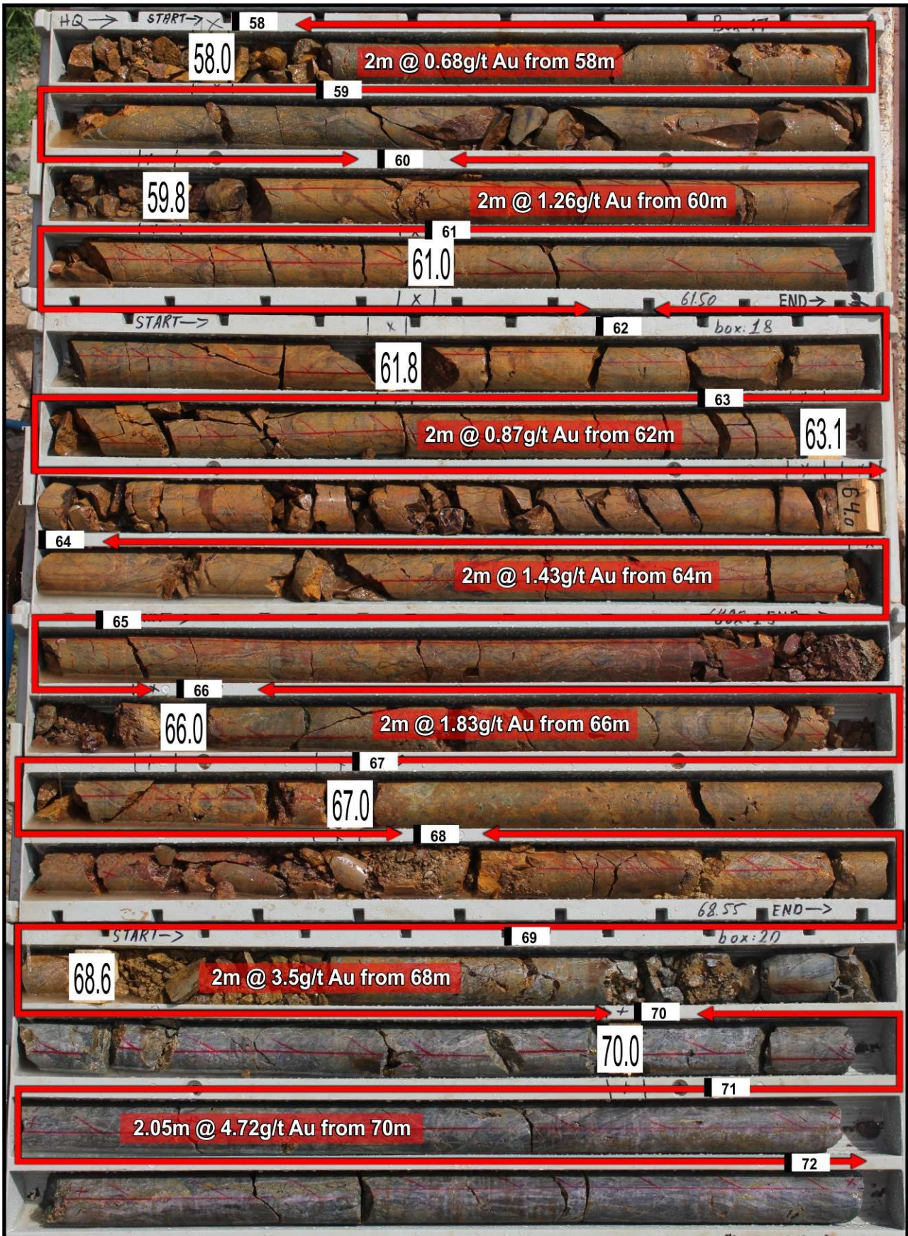
FIGURE 10: Drill core from Copper Hill demonstrating high-grade oxide material.
