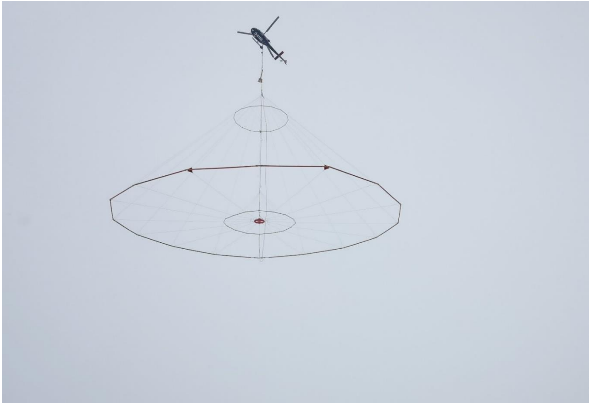
Figure 5: VTEM™ Max System deployed over the Zeus Project Areas
