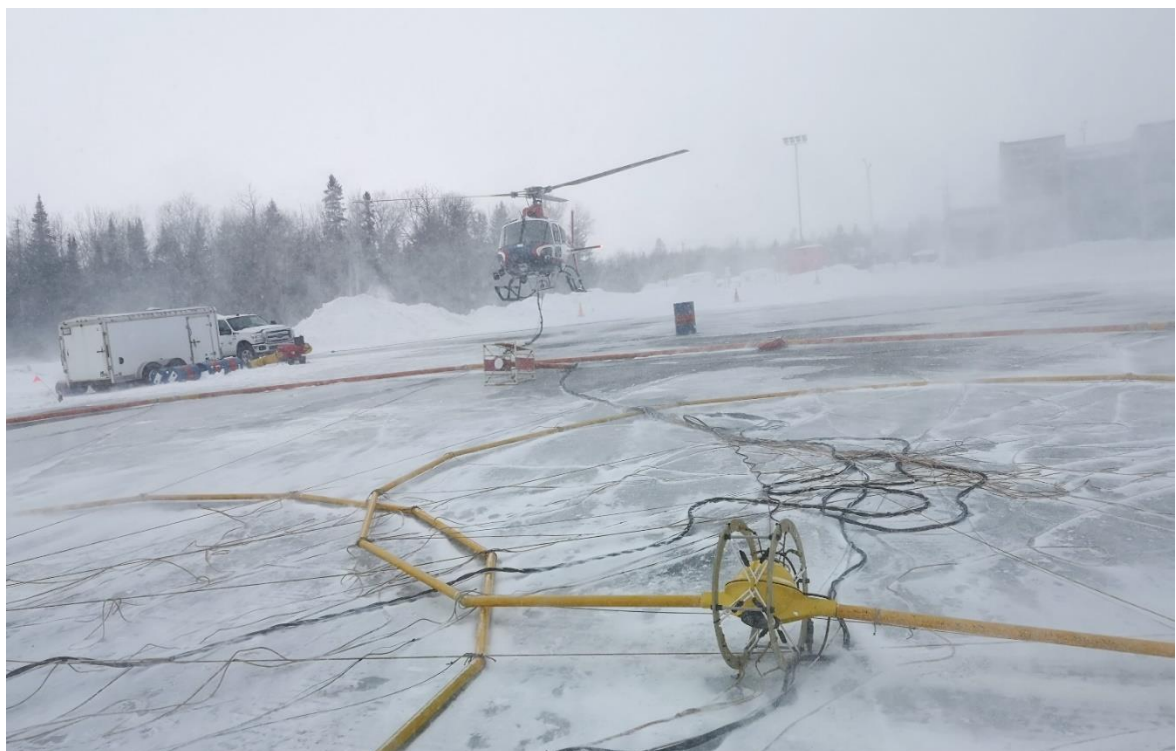
Figure 6: Geotech crew 'landing' the 35m diameter transmitter loop Saint Bruno Airport.
