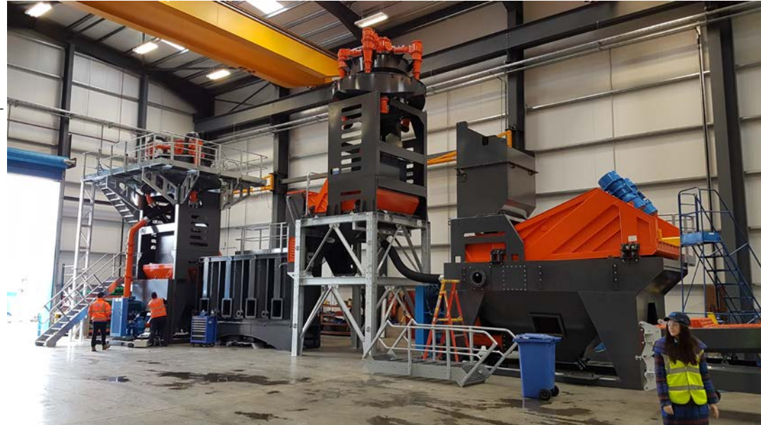
Start-Up 70tph modular wet plant
