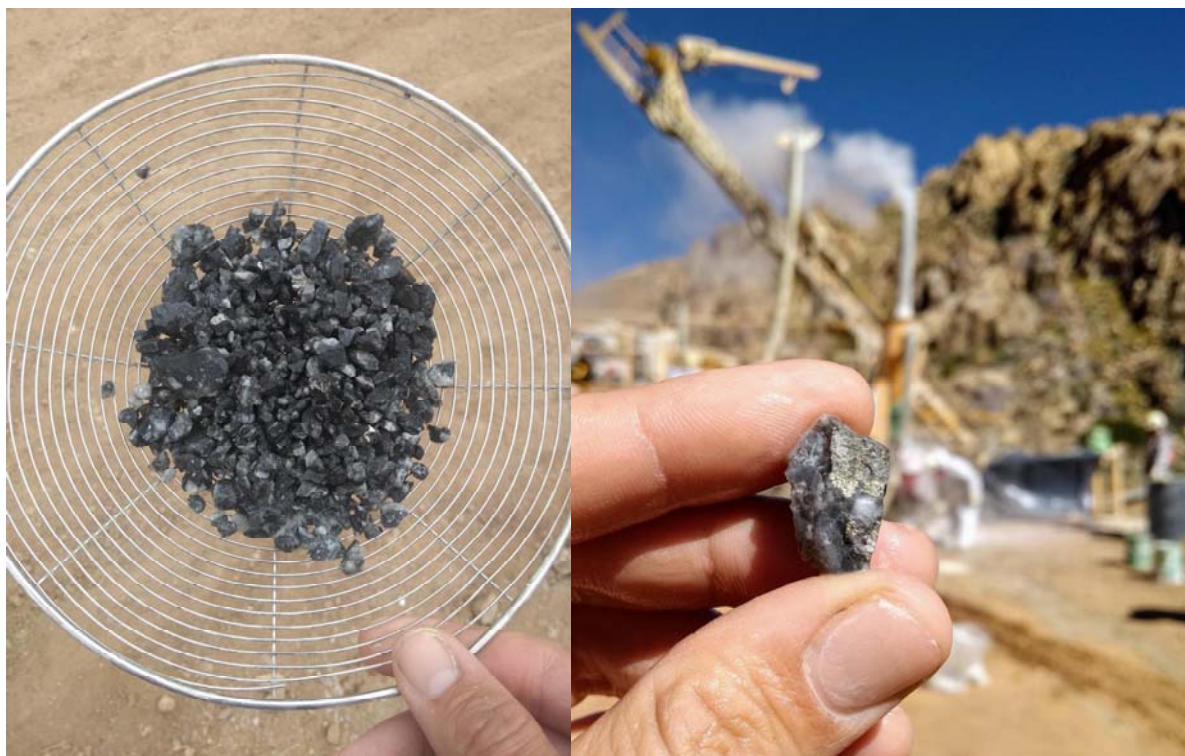
Photo 5 (left): LORC19-07, Tramway Target vein. Sulfides in chalcedonic quartz vein-breccia: pyrite, sphalerite, arsenopyrite. Photo 6 (right): LORC19-07, Tramway Target vein. Chalcedonic quartz vein with some brecciation: red sphalerite, pyrite, some chalcopryite.
