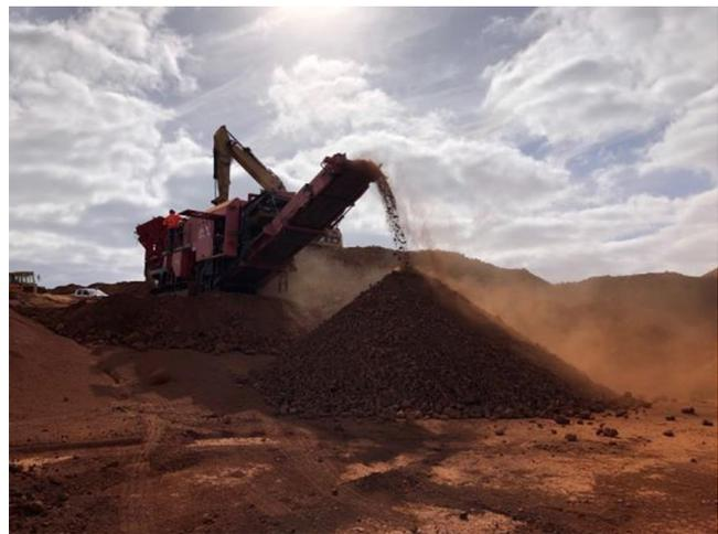
**Figure 2: Bauxite product from crusher-screen**
