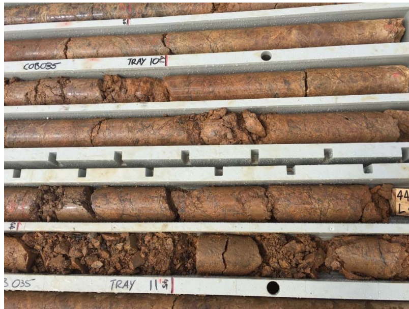
Figure 4 – Drill core (COB035) highlighting shear zone (fractured zones)
