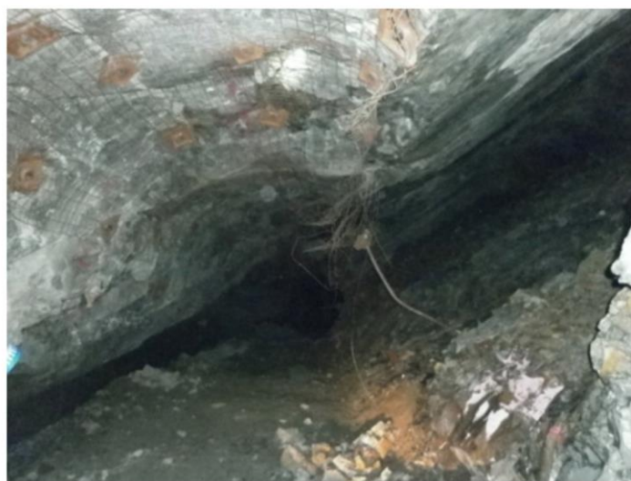
ABOVE: A mined area from Citigold's test mining showing the floor of the level drive, and the stope voids (ore extracted area) above and below the level. The ore has been cleanly extracted, showing how the mining method minimizes dilution by maintaining a marrow stoping 'slot' width.
