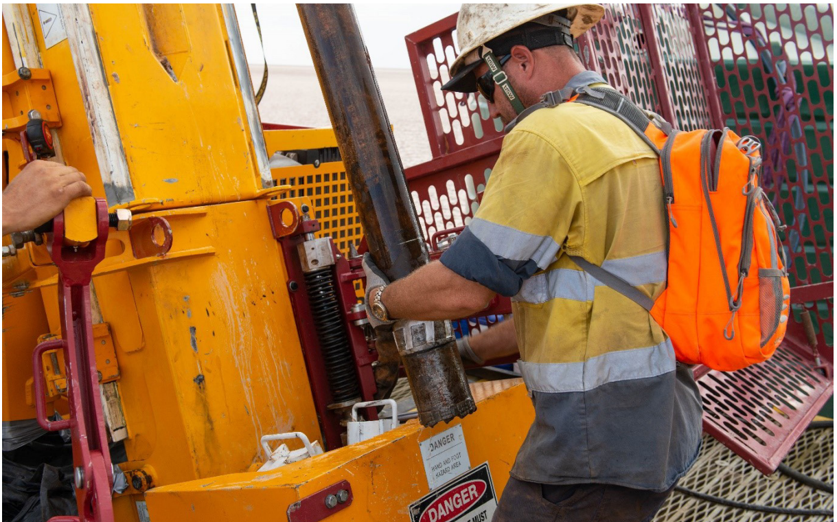
Photo 4 A driller inserts a diamond drilling bit at drillhole TD7, January 2019.
