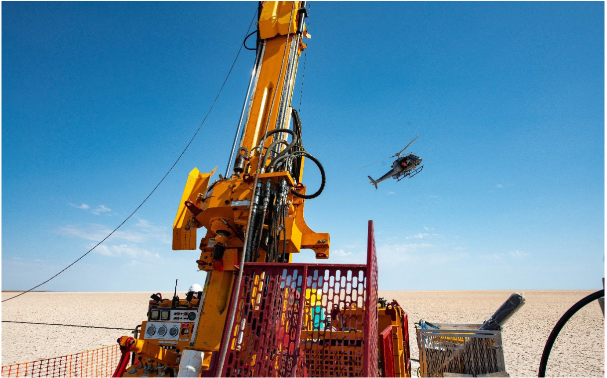
Photo 3 Lake Torrens drilling is helicopter supported to avoid heavy vehicle traffic on the salt lake crust, January 2019.
