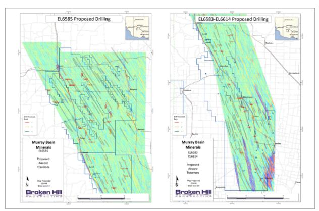
Figure 2. Interpreted magnetic anomalies for the Ouyen and Tyrrell Ridge HMS districts with high priority drill traverses.
