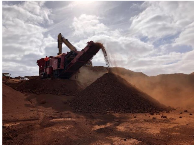
Figure 4: Bauxite product from crusher-screen
