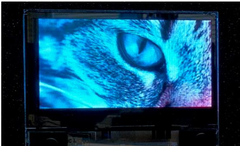
X-Celeprint 2000 cd/m 2 microLED display, using RPCVD p-GaN, showing good colour uniformity quantum efficiency and forward voltage
